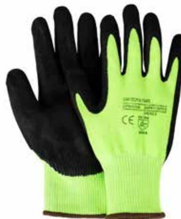
High visibility HPPE glove coated with NBR foam and sandblasted palm. EN420, EN388, Level 5
